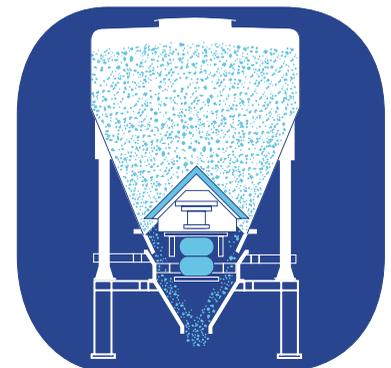
3. Cone valve lifts and vibrates to discharge materials as required.
